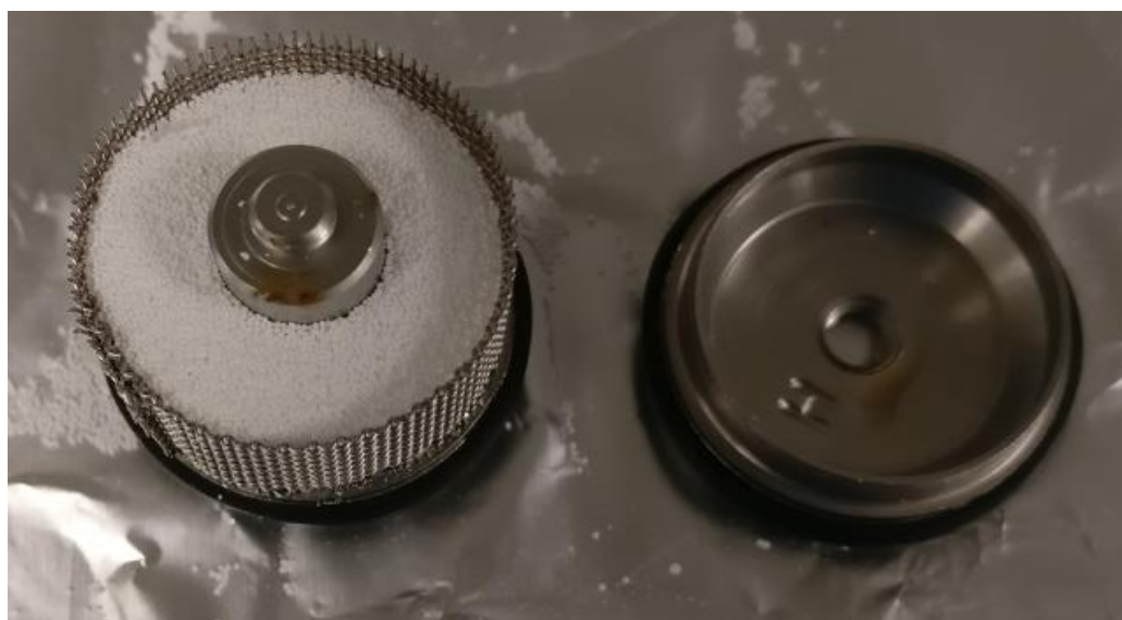
Figure 6.14. Particle size distribution of ECR8204F and ECR8204M enzyme immobilization resins and photograph of the resin in an ACR catalyst basket. Resins were analysed by laser diffraction as described in Section 2.4.3.2. The catalyst baskets have a mesh with an approximate pore size of 400 µm and are approximately 2.5 cm across.
