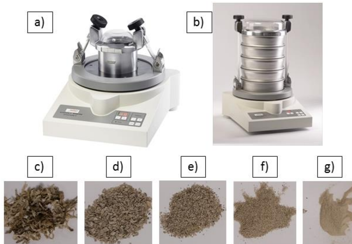
Figure 2.2. Ball mill and sieve set up and SBP fractions. Ball mill (a) and sieve (b) setup used for milling and sieving dry SBP. Images below show samples of the dried and sieved SBP: (c) dried cossettes ; (d) milled SBP larger than 1 mm; (e) milled SBP larger than 500 \mu\text{m} and smaller than 1 mm; (f) milled SBP larger than 212 \mu\text{m} and smaller than 500 \mu\text{m} ; and (g) milled SBP smaller than 212 \mu\text{m} .
