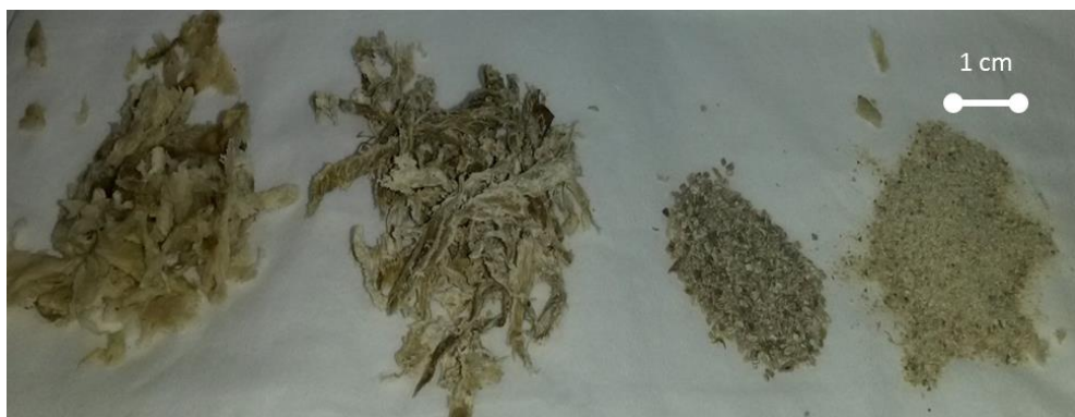
Figure 1.6. Photograph of different forms of SBP. From left to right: wet SBP from diffuser; dried SBP; coarsely ground dry SBP to >0.5 mm; and milled SBP to <0.5 mm. Scale bar is 1 cm.
