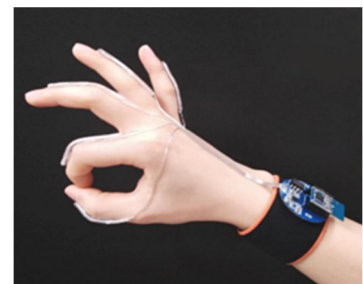
A translation device with stretchable sensor arrays on each finger attached to a wireless circuit board on the wrist. Image from (Zhou et al., 2020) (permission requested).
