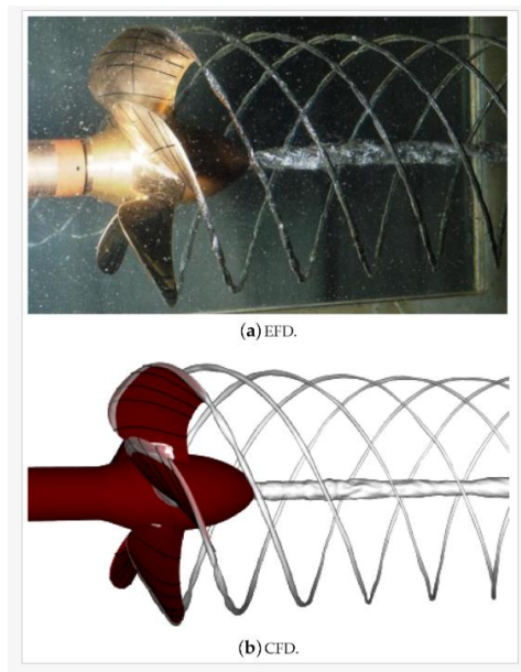
702 Figure 23: Tip and hub vortex structures during (a) experiments and (b) DDES computations. (Viitanen et 703 al., 2018)
