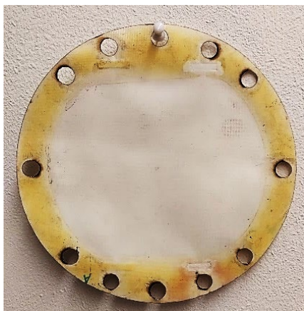
Figure 27. Zirfon Perl, photo Nick Laessing
