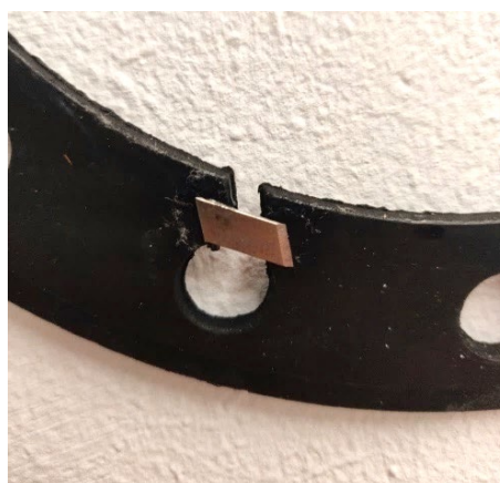
Figure 28. Gasket detail with cutter blade, photo Nick Laessing
