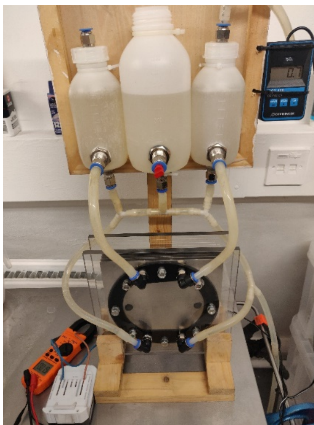
Figure 25. Two-plate electrolyser, photo Nick Laessing
