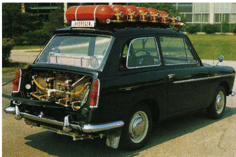
Figure 56. Karl Kordesch's 1970 Hydrogen Fuel Cell Car. Used for over three years as daily transportation. . Karl Kordesch, Industrial and Engineering Chemistry 52:4 (1960), pp. 296-298; Kordesch K.: Fuel Cells and their application , Weinheim VCH 1996
