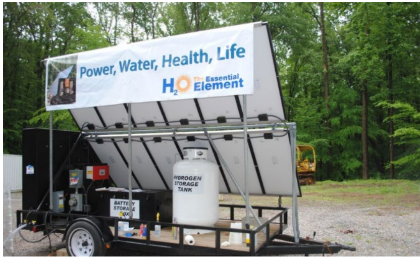
Figure 54. Mike Stritzki's Hydra solar hydrogen mobile generator and water purifier "Hydrogen House Project: Hydra Water Purifier," Hydrogen House Project , accessed April 23, 2021, https://hydrogenhouseproject.org/hydra-mobile-generator--water-purifier.html .
