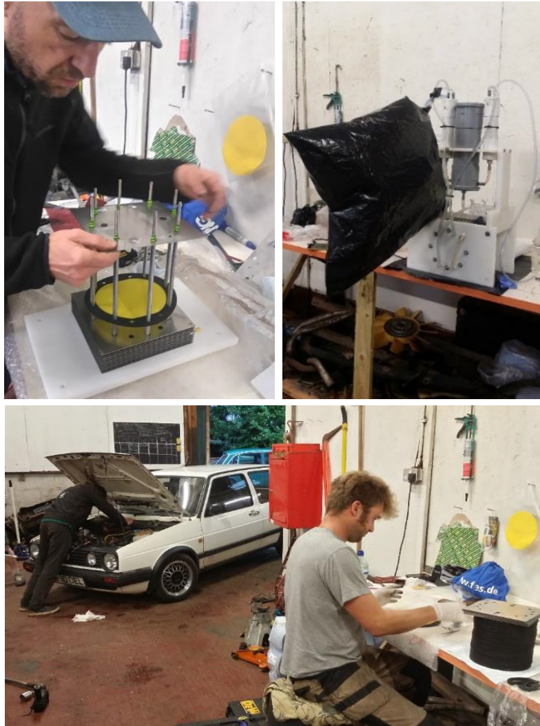
Figure 21. Water Gas Car Workshop fabrication using polyester silk screen printing fabric for gas separation membranes, Nick Laessing (top), Jimmy Whitmore (left) and Jonah Kinross (right), Devon, photo Nick Laessing, Jonah Kinross.
