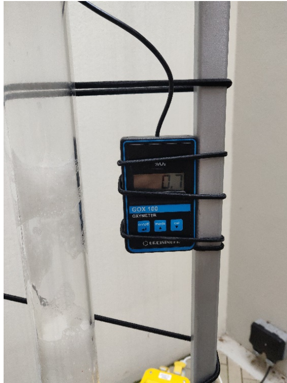
Figure 35. Gas analyser showing 0.7% O 2 , or 99.3% H 2 . photo Nick Laessing
