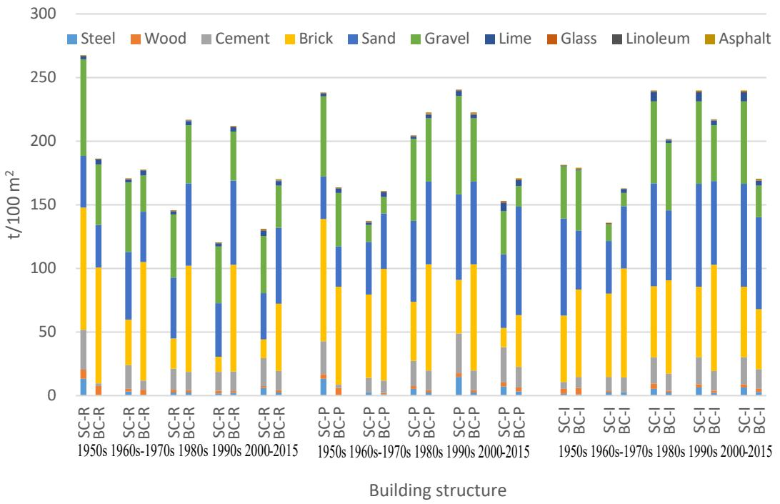
**Fig. 6.** The comparison of material intensities between steel-concrete and brick-concrete buildings.
