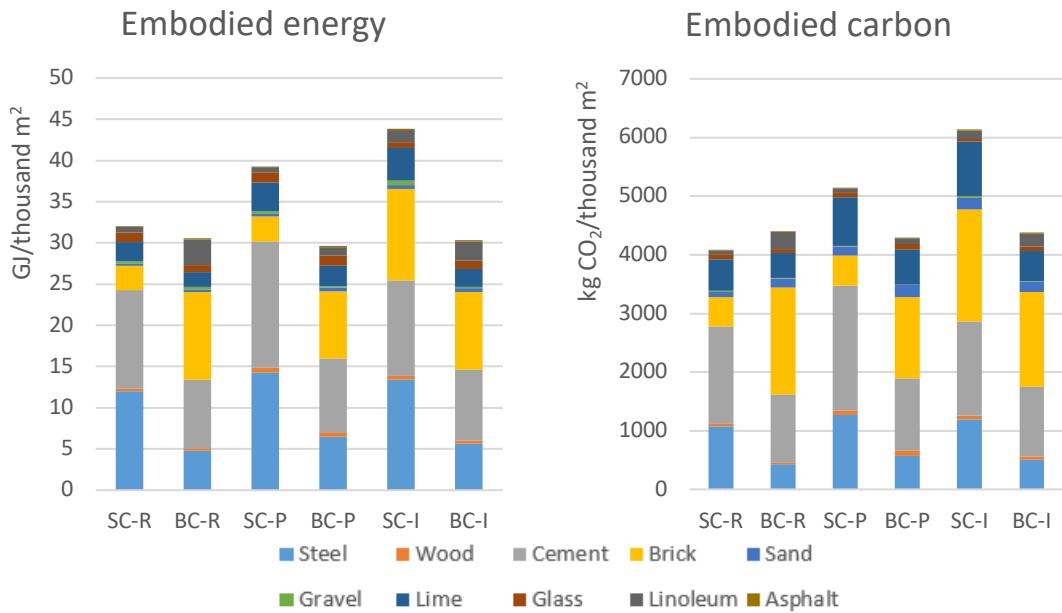
**Fig. 7.** The comparison of embodied energy and carbon between steel-concrete and brick-concrete buildings (2018).
