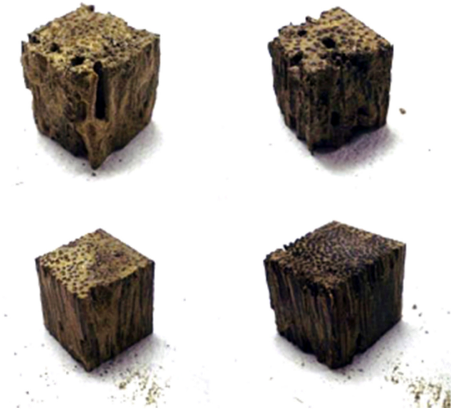
Figure 8: OPW after cleaning at the end of the termite test. Top left: untreated OPW; top right: treated OPWD-0%; bottom left: treated OPWD-25%; and bottom right: treated OPWD-50% [76].
