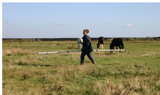
Fig 3.5 Photograph of EM 31 geophysical survey in progress
