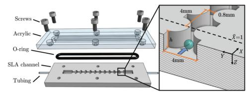
Figure 4. Schematic of a millifluidic porous medium used to study deformable particle transport. Reproduced from M G O'Connell *et al* 2019 with permission of The Royal Society of Chemistry.
