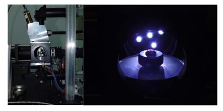
**Figure 3.** The aerodynamic levitation furnace installed at Wuhan University of Technology. Left shows the sample cell with heating lasers supplied top and bottom and shadow casting laser supplied from the left. Photo on the right shows nozzle jet with sample illuminated by low power alignment lasers. Photo credit D Langstaff (c) 2015.
