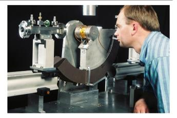
**Figure 1.** A combination of QuEXAFS and powder diffraction installed on beamline 9.3 of the SRS in Daresbury. This was a prime example of technique combinations used in time-resolved experiments. The high temperature furnace was developed in the Royal Institution. Above the furnace the measuring head of the 13-element monolithic Ge fluorescence detector can be seen. The curved INEL detector was used to collect powder diffraction data at the same time. Photo credit: STFC.
