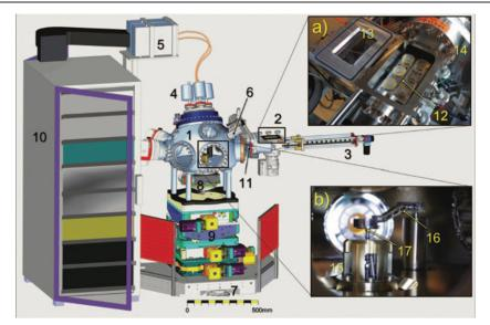
**Figure 5.** Overview of the highly automated sputter equipment. Reprinted from R Dohrmann *et al* 2013 with the permission of AIP Publishing.
