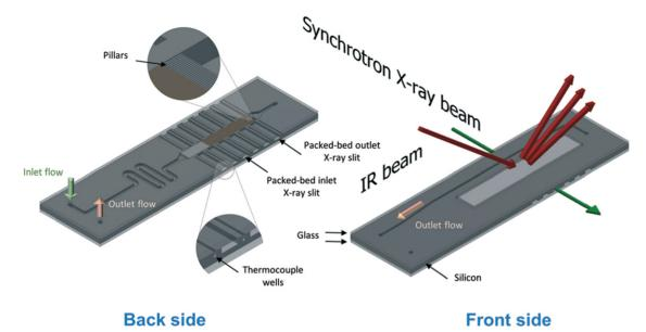
**Figure 6.** Schematic representation of the back and front side of the microreactor for operando XAS/MS and DRIFTS/MS studies. A packed-bed catalyst (brown) and glass beads (light grey) upstream of the catalyst bed are depicted on the back side image. Insets show detailed view of the pillars used for retaining the catalyst particles and the thermocouple wells. Reproduced from B Venezia *et al* 2020. CC BY 3.0.
