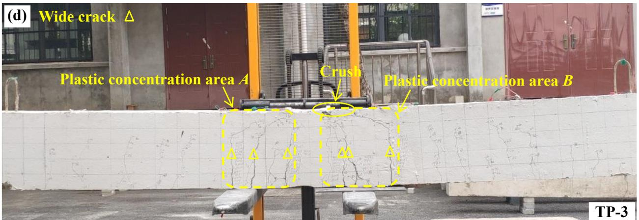
Fig. 10. Failure modes of specimens under three-point bending: (a) TC-C; (b) TP-1; (c) TP-2; (d) TP-3.
