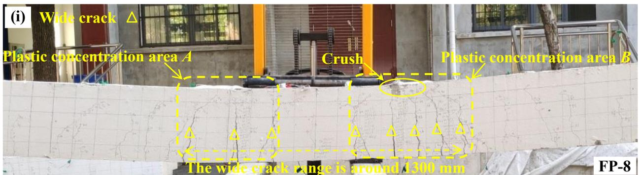
Fig. 16. Failure modes of specimens under four-point bending: (a) FC-C; (b) FP-1; (c) FP-2; (d) FP-
