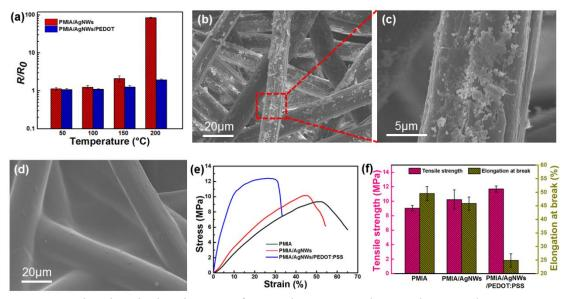
Figure 5. The electrical resistance of PMIA/AgNWs and PMIA/AgNWs/PEDOT:PSS
