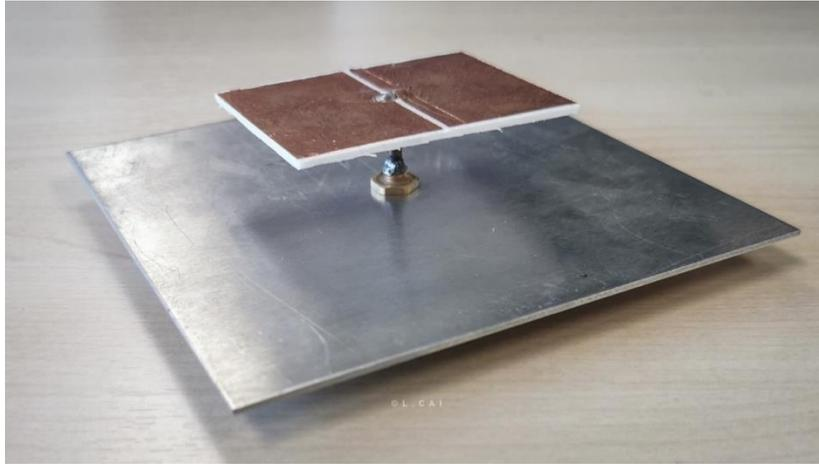
Fig. 3.15: The photography of fabricated cavity-less Pseudo-ME dipole prototype
