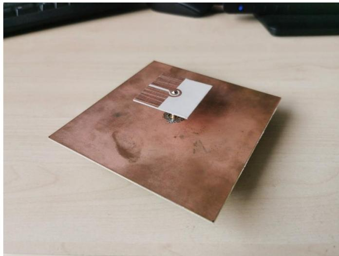
Fig. 4.31: The fabricated CP Pseudo-ME dipole antenna
