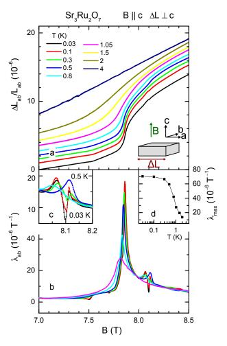
**Figure 2** a: Linear magnetostriction  $\Delta L_{ab}/L_{ab}$  of Sr<sub>3</sub>Ru<sub>2</sub>O<sub>7</sub> measured perpendicular to the *c*-axis at various temperatures for  $B \parallel c$ , as indicated in the sketch. b: Respective magnetostriction coefficient  $\lambda_{ab}(B)$ . Inset c enlarges region close to upper metamagnetic transition. Inset d displays temperature dependence (on a log scale) of maxima in  $\lambda_{ab}$  at the central metamagnetic transition.
