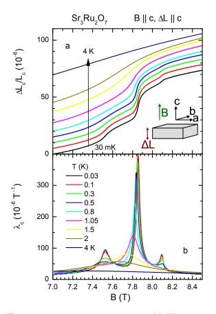
**Figure 1** a: Linear magnetostriction  $\Delta L_c/L_c$  along the *c*-axis of Sr<sub>3</sub>Ru<sub>2</sub>O<sub>7</sub> measured at various temperatures for  $B \parallel c$ , as indicated in the sketch. b: Respective magnetostriction coefficient  $\lambda_c(B)$ .
