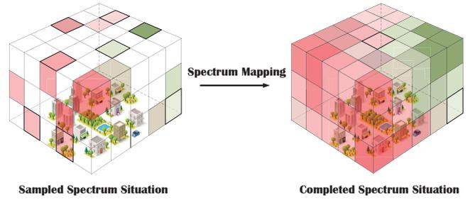
Fig. 2. Graphical illustration of 3D spectrum mapping. It aims at accurately recovering the situational values of all locations in the entire 3D space through a small number of sampling points.
