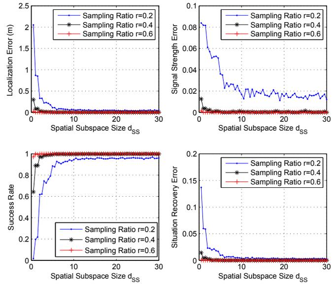
Fig. 10. Impact of spatial subspace size  $d_{SS}$  on the QR-3DOMP performances of localizations, signal strength recovery, success rate and spectrum situation recovery ( $r = 0.2, 0.4, 0.6$ ).
