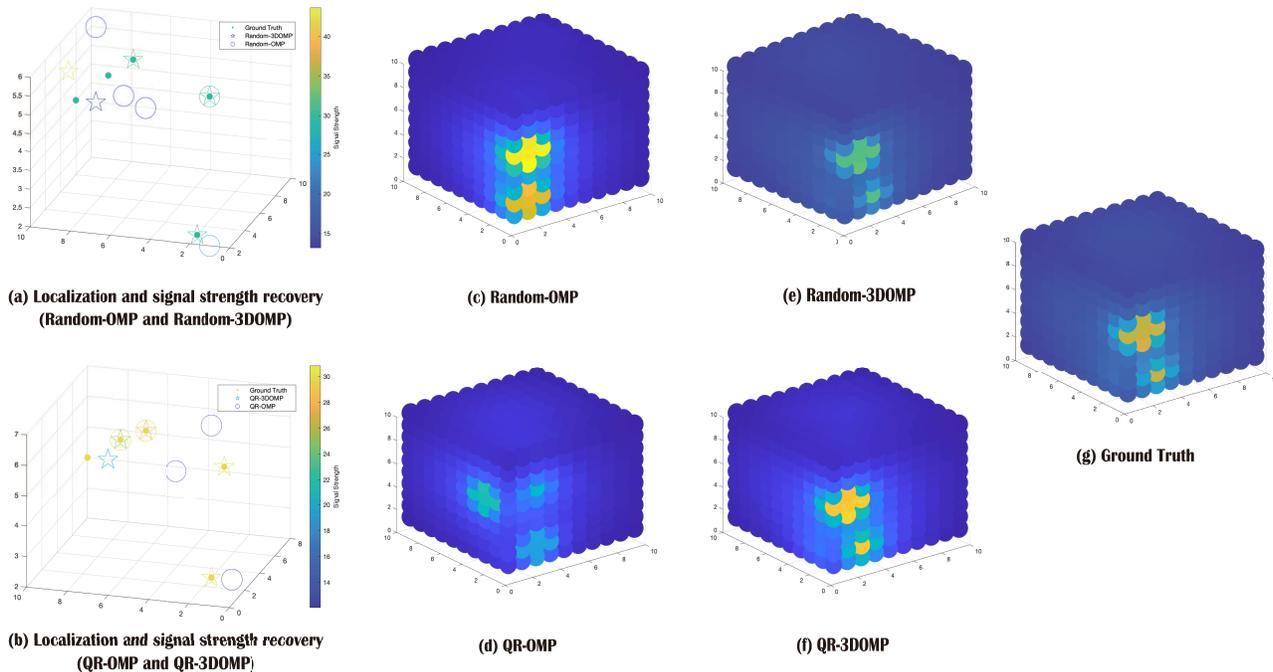
Fig. 15. 3D spectrum mapping performance visualization ( $r = 0.1$ ,  $d_{SS} = 3$ ). (a) and (b) present the localizations and signal strength recovery of Random-OMP, Random-3DOMP and QR-OMP, QR-3DOMP, respectively. (c), (d), (e) and (f) show the spectrum situation recovery. (g) is the ground truth of spectrum situation.
