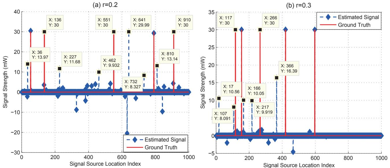
Fig. 4. Sparse signal  $\mathbf{x}$  recovery performance with random sampling matrix  $\phi$  and traditional OMP recovery algorithm. The sampling rates are 0.2 and 0.3 for (a) and (b) respectively. It is observed that the estimated signal source locations and signal strengths are not accurate, however, the estimated locations are always adjacent to the real signal sources in the Cartesian coordinate.
