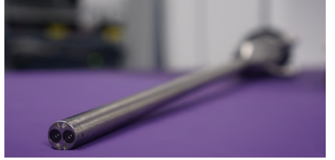
Fig. 3. The 0 degree scope used in the experiment. The kinematic chain defined in Eq. 4 assigns the final frame at the centre of the tip of the scope (ECM frame), which is not the same as the camera position and orientation. The CAM frame is typically defined at somewhere in front of the scope, and hand-eye calibration is the process to identify the exact pose of the CAM frame.
