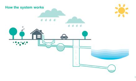
Fig. 25.4: How the tunnel will work. Source: Image courtesy of Thames Tideway.
