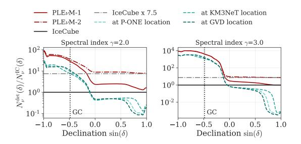
**Figure 2:** Number of neutrinos detected by all constituent detectors and PLE $\nu$ M-1/2 for through-going muon tracks relative to neutrinos detected by IceCube at the respective sine of declination. The two plots show the ratio calculated based on spectral indices of  $\gamma = 2.0$  and  $\gamma = 3.0$  of the astrophysical neutrinos. The declination of the Galactic Center is marked with a vertical, dotted line.
