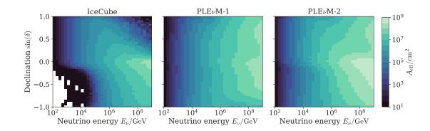
**Figure 1:** Comparison of the effective area for through-going muon tracks of IceCube, PLE $\nu$ M-1 and PLE $\nu$ M-2 as a function of energy and sine of declination. PLE $\nu$ M-1 consists IceCube and IceCube-like detectors at the locations of P-ONE, KM3NeT and Baikal-GVD. For PLE $\nu$ M-2, we assume a detector that is 7.5 times larger than IceCube instead of IceCube's contribution to PLE $\nu$ M.
