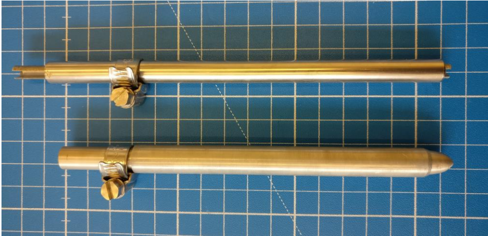
Figure 3: Prototype of the implantation tool made of a trocar with dilation tip (lower part), and the electrode delivery tool (upper part).
