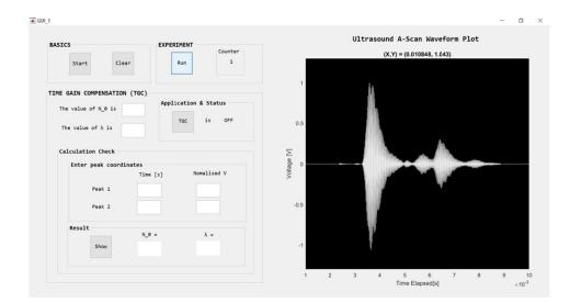
**Figure 1.** The user interface developed in MATLAB R2018a using the in-built GUIDE function. There is a control panel on the left-hand size and a display of the waveform on the right-hand side (voltage/amplitude against time).
