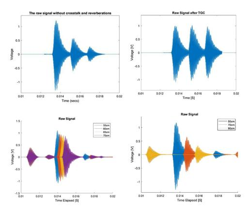
**Figure 4.** (a) (top left) The waveform plot before applying TGC algorithm. (b) (top right) The waveform plot after applying TGC algorithm. (c) (bottom left) The waveform plot showing resolvable peaks. Here the distance *D* between adjacent positions of the phantom is 20 cm and this is larger than the axial resolution of the range finder. (d) (bottom right) The waveform plot showing unresolvable peaks, with D = 5 cm (D < axial resolution).
