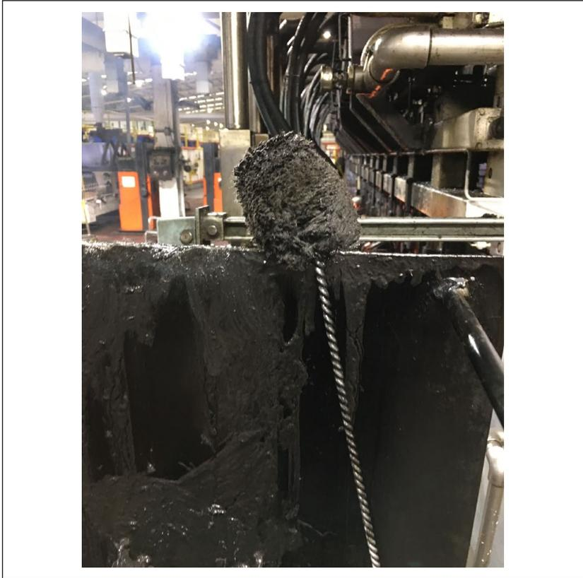
**Figure 1.** A swabbing brush/stick used to apply oil (dobe) to the molds in the machinery that can be seen in the background of this photo.
