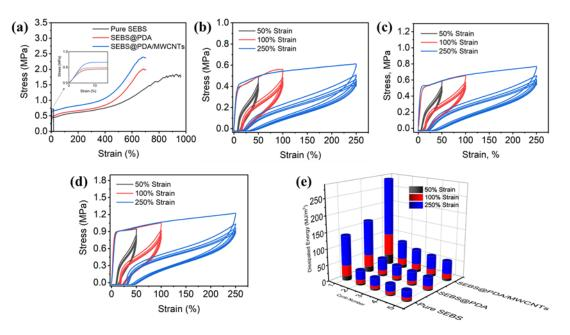
Figure 6 Stress-strain curves of pure SEBS, SEBS@PDA, and
