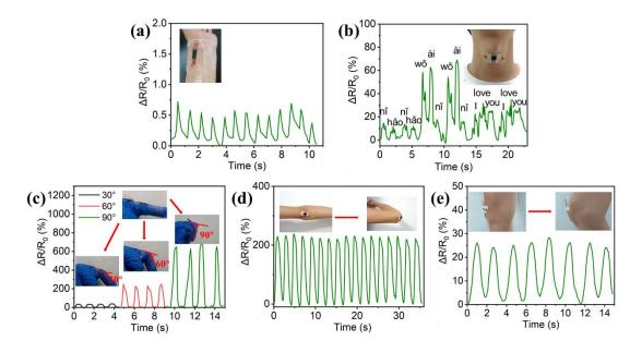
Figure 11 Strain sensors used to monitor human motions. (a) pulse beat, (b) vocal cord vibration, (c) finger bending, (d) elbow bending, (e) knee bending.
