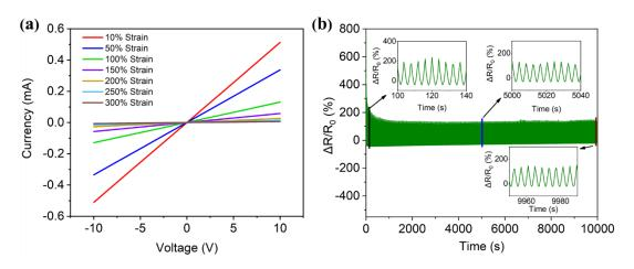
Figure 9 (a) Current and voltage of fiber composites under different strains of 10%, 50%, 100%, 150%, 200%, 250%, and 300%. (b) 2500 cycles at 0–40% strain at a
