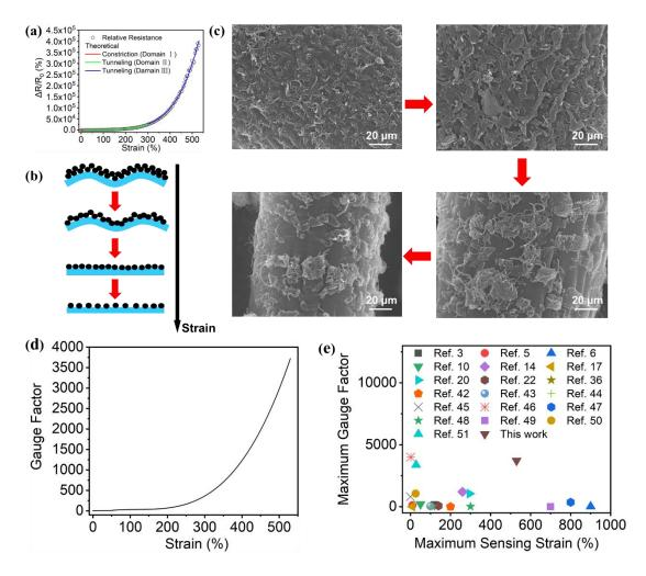
Figure 7 (a) The relative resistance–strain curve of fiber composites at a stretching rate of 10 mm/min. (b) The schematic illustration of longitudinal sections of fiber composites during stretching. (c) The SEM images of fiber surface during stretching.
