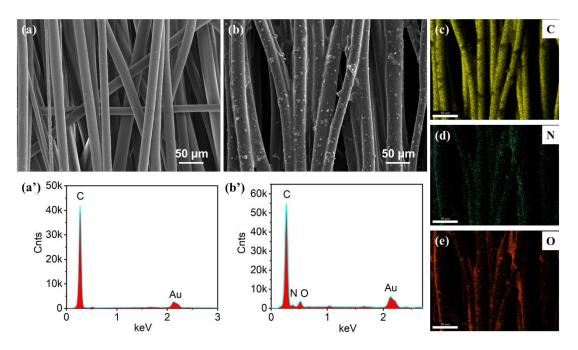
Figure 2 SEM images and EDX spectroscopy of (a), (a') pure SEBS and (b), (b') SEBS@PDA, respectively. EDX mapping images of SEBS@PDA for (c) C, (d) N,
