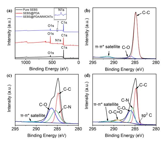
Figure 4 (a) XPS wide scan spectra of pure SEBS, SEBS@PDA and
