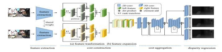
**Fig. 1**. Diagram of our proposed network. Our network architecture consists of four modules: feature extraction, cost construction, cost aggregation and disparity regression. In the cost construction, we propose two new feature wrangling ideas: (a) spatially a differentiable feature transformation; (b) channel-wise a memory-economical feature expansion. Moreover, in the cost aggregation, we also revamp the connections between 3D convolutions.
