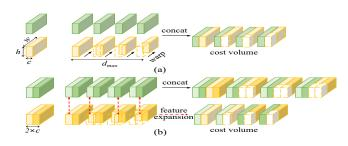
**Fig. 4.** (a) Conventional feature volume construction by concatenating cubes of c features from the left (green) and shifted right (yellow) views. (b) (lower) Our feature expansion vs. (upper) concatenation of cubes of kc features (divided into k subsets of c features) for feature volume construction. k = 2 and  $d_{max} = 4$  are used in illustration.
