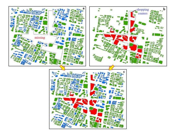
Fig. 2. Building footprint determination process (a: extracted building footprints from BDM;b: extracted building footprints from OSM; c: combination of a and b).
