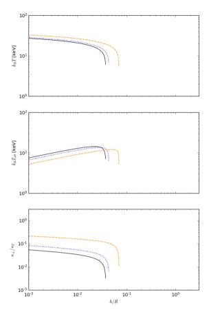
**Figure 8.** The accretion column properties for the same set of models as in Fig. 7. From top to bottom, the plots show the central internal temperature profile, the effective temperature profile of the emitting radiation, and the perpendicular mean opacity, respectively.
