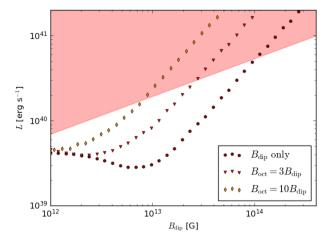
**Figure 10.** Maximum luminosity against surface dipole field strength. The red-shaded region indicates the region for which *L* exceeds the NS Eddington luminosity at the magnetospheric boundary, i.e. when the accretion flow is super-Eddington. The circles, the triangles, and the diamond points show the computed maximum luminosity for a pure dipole, a  $B_{\text{oct}} = 3B_{\text{dip}}$ , and a  $B_{\text{oct}} = 10B_{\text{dip}}$  surface magnetic field configuration, respectively.
