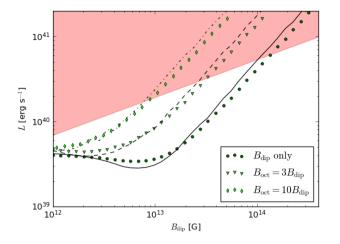
**Figure 11.** Same plot as in Fig. 10 for models with different polarization fraction. The circles, the triangles, and the diamonds in green are computed using f = 0.7, and assuming a pure dipole, a  $B_{\text{oct}} = 3B_{\text{dip}}$ , and a,  $B_{\text{oct}} = 10B_{\text{dip}}$ , surface magnetic field configuration, respectively. The solid, dashed, and dot-dashed black lines shows the same configurations but computed with f = 1.
