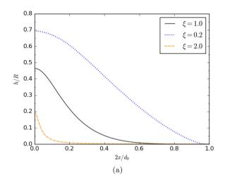
**Figure 6.** Half vertical cross-section of the sinking region for models with  $L_{39} = 1.0$ ,  $B_{dip} = 3 \times 10^{12}$ G, and  $B_{oct} = 0$ . The different curves correspond to different values of the power law index:  $\xi = 1$  (the black solid line),  $\xi = 0.2$  (the blue-dotted line), and  $\xi = 2$  (the orange dot–dashed line).
