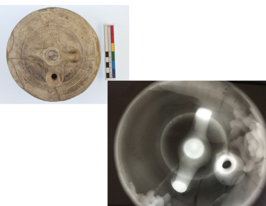
Figure 4. Ceramic stirrup jar from Tell el-Ajjul (Palestine) as reconstructed in visible light (left) and x-radiograph of jar showing application method used in loss compensation (UCL-IoA EXIII.57/1)
