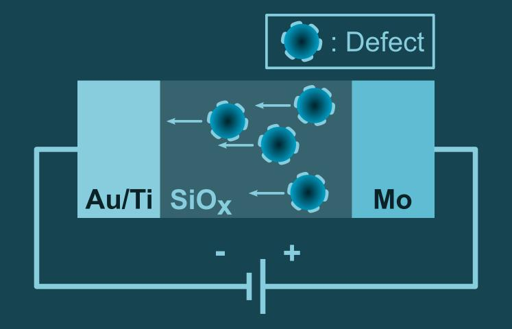
One possible method to observe vacancy properties is via a phenomenon called the current transient – a characteristic current time response with a prominent current peak.
