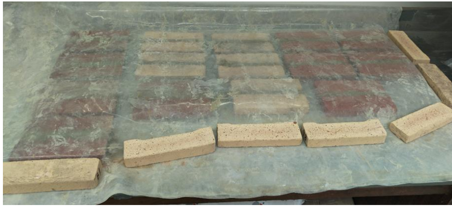
Figure 7: Bonded samples, mortar cubes and vapour barrier
