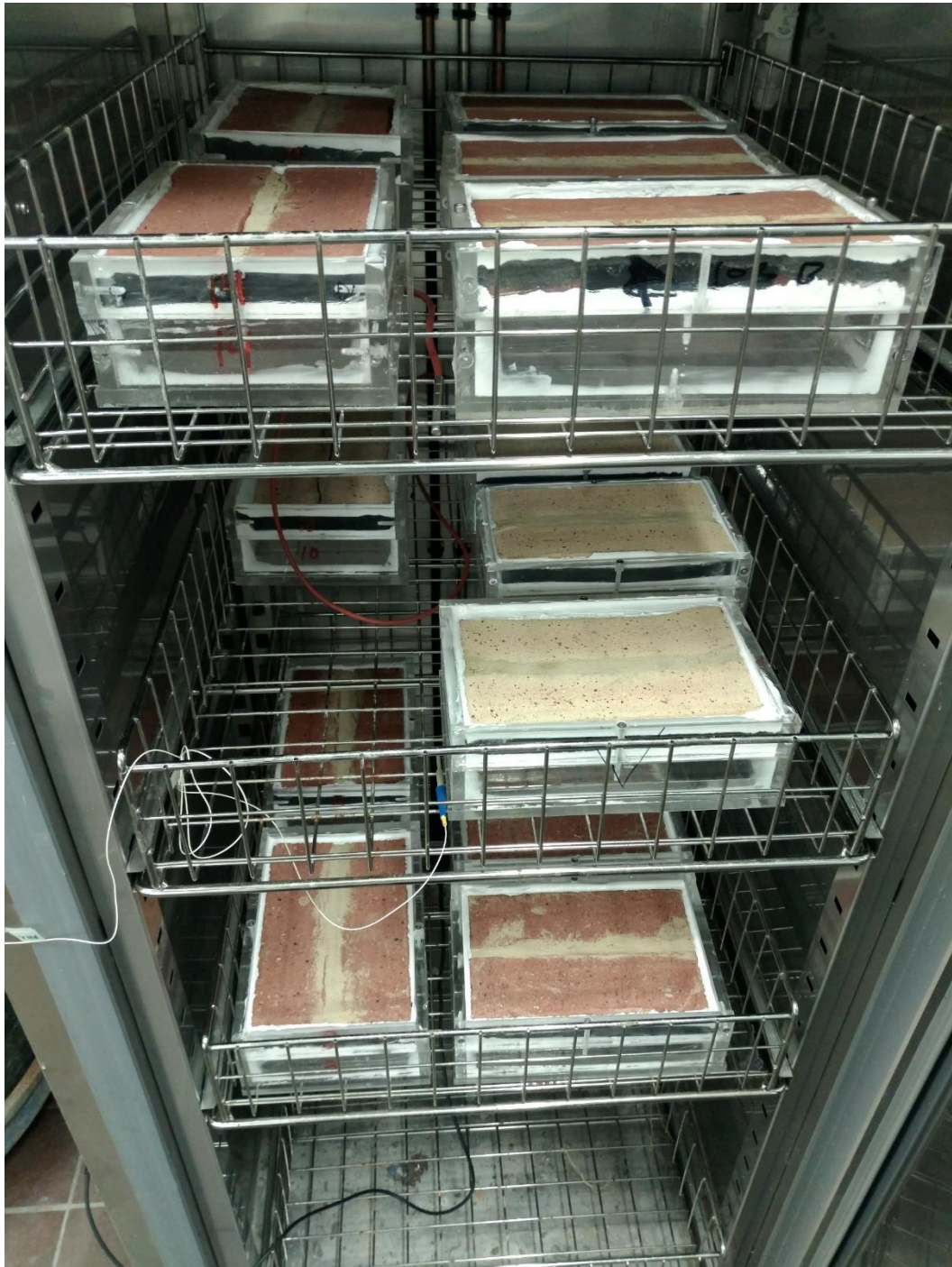
Figure 13: Humidity and temperature control chamber with testing boxes
