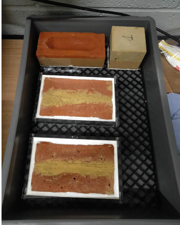
Figure 15: Three different types of specimens during absorption test
