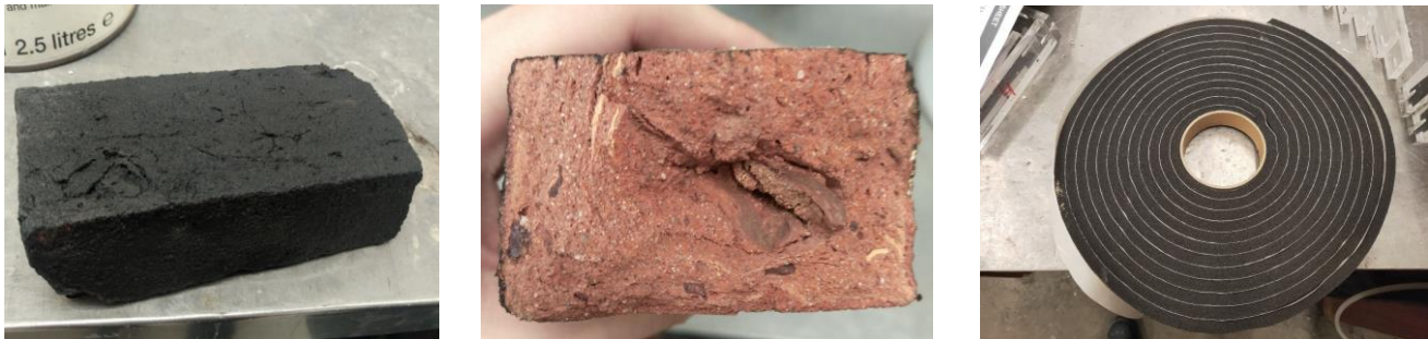
Figure 10: a) Adhesive over the brick surface; b) cross section penetration; c) foam tape
