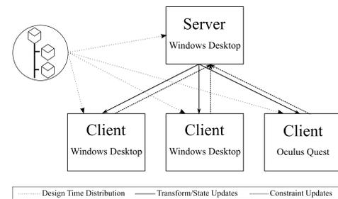
Fig. 3: Message flow diagram of edge-physics network
