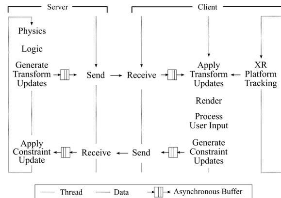
Fig. 1: Logical flow diagram for prototypical implementation
