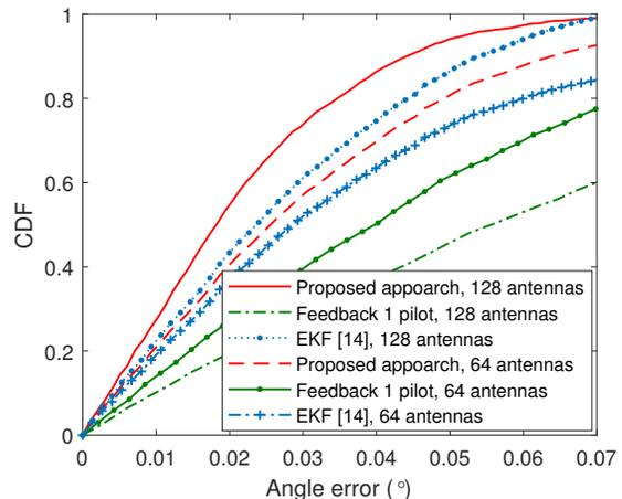
Fig. 10. CDF of the angle estimation error.
