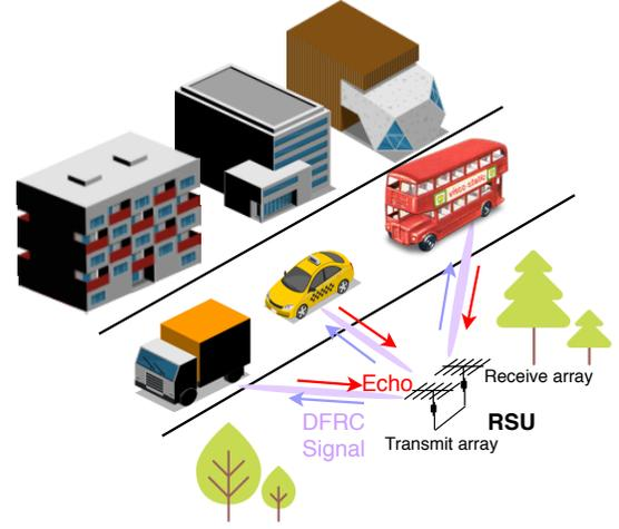
Fig. 1. System model for the considered vehicular network.
