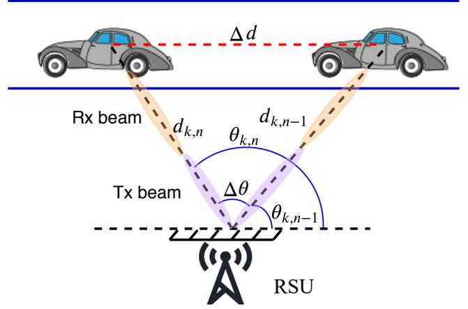
Fig. 2. State evolution model of the considered vehicular network.
