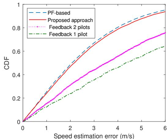
Fig. 9. CDF of the speed estimation error.
