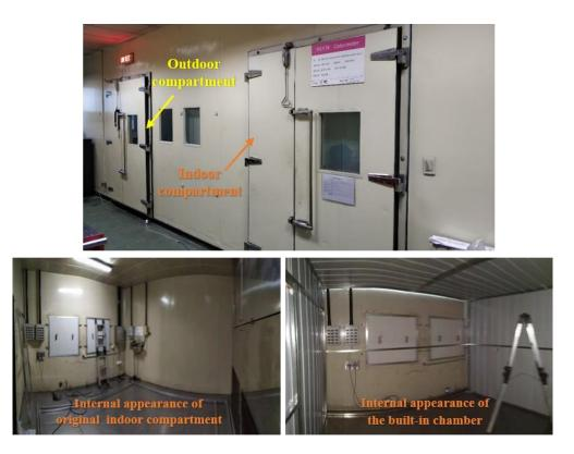
Fig. 1. The prototype of the calorimetric chamber.
