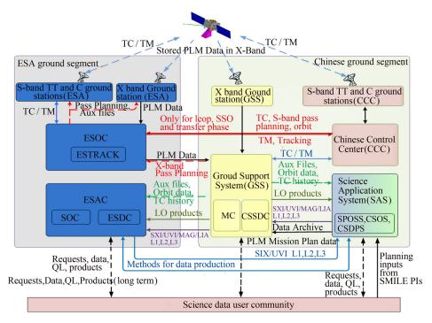
Fig. 7 Ground segment block diagram of SMILE mission
