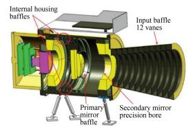
Fig. 3 Structure diagram of UVI
