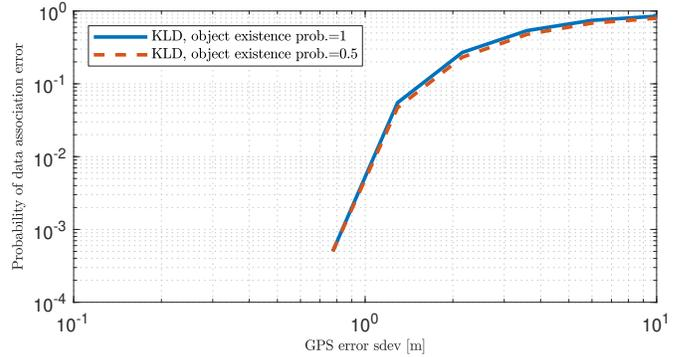
Figure 3. Probability of data association error for the scenario with 20 vehicles and 20 objects for changing GPS error standard deviation.
