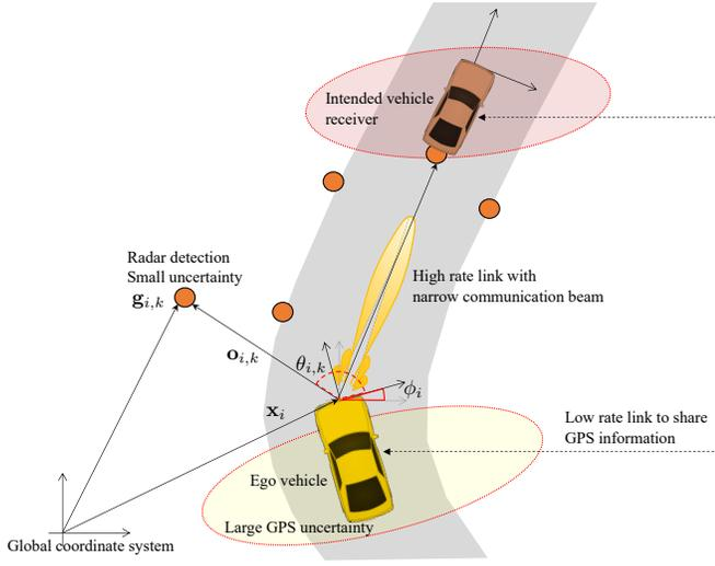
Figure 1. Scenario: the ego vehicle has unknown location and heading. It measures objects using a radar in its local frame of reference.
