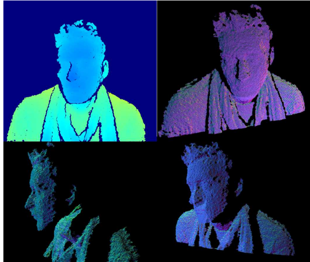
Figure 2. Example of high quality depthmap and point clouds generated with HashMatch. Notice the level of details and the absence of quantization and outliers.
