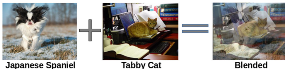
Fig. 7 An example of how blended images are created. Images from two categories are alpha-blended—each component image’s pixel value is reduced by 50% and added into one image
