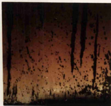
Figure 4.10b The textures of SCE12 aligned in a polyimide wedge cell 0-6 \mu\text{m}
