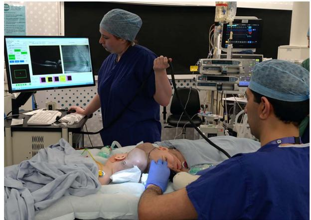
**Figure 4:** Handheld OCT acquisition. OCT image acquisition in lateral decubitus position under general anaesthesia using handheld OCT device.
