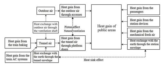
Figure 1: Schematic of heat gains for the public areas of typical underground stations.
