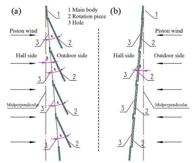
Figure 7: The new type of door curtain and its resistance component: (a) Train arriving station, (b) Train leaving station (adapted from [53]).
