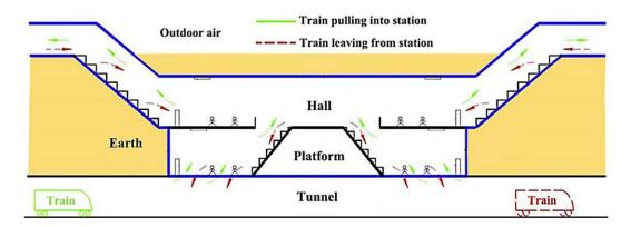
Figure 5: Air flow schematic of the piston effect in an island-type station (adapted from [53]).
