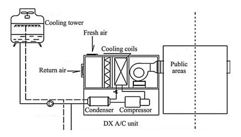
Figure 10: A schematic diagram for DX A/C systems.
