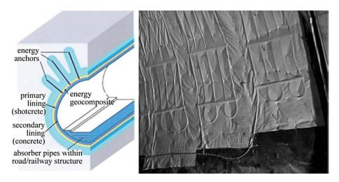
Figure 13: Schematic of an energy tunnel (adapted from [97]).
