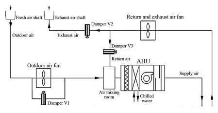
Figure 8: Air flow pattern in ventilation systems.
