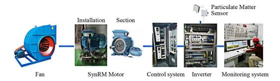
Figure 9: Ventilation system with inverter equipped in metro stations (adapted from [66]).
