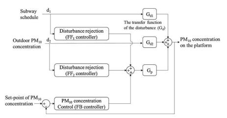
Figure 11: Block diagram of the ventilation control system for the metro station
