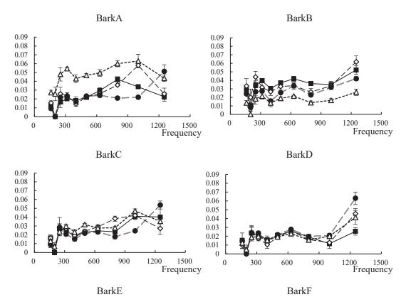
Fig. 3 The absorption coefficient of 4 bark samples taken at different positions along the trunk circumference, for the 6 species considered.
