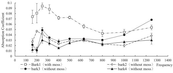
Fig. 5 The difference of absorption between bark with moss and without moss
