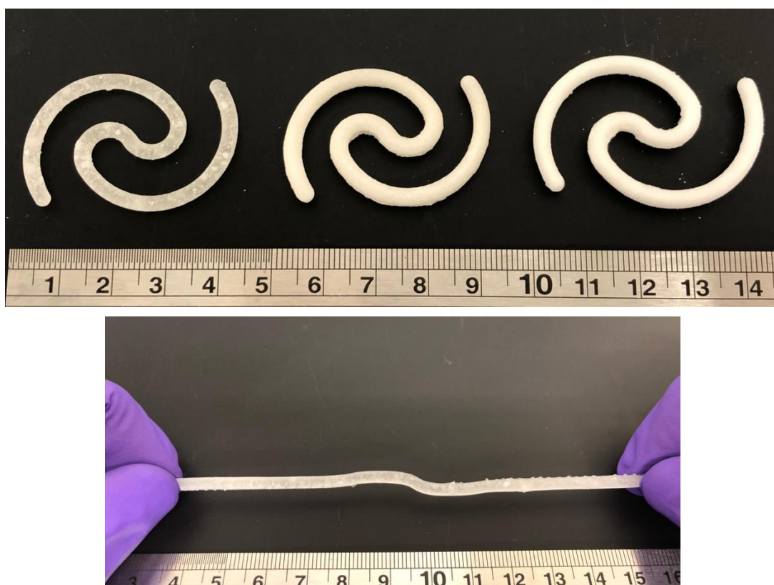
Figure 6. Photograph of the SLA 3D printed solid 10% device (top left), solid 30% device (top middle), and solid 50% device (top right) bladder devices and the solid 10% device under stretching (bottom). Scale in cm.
