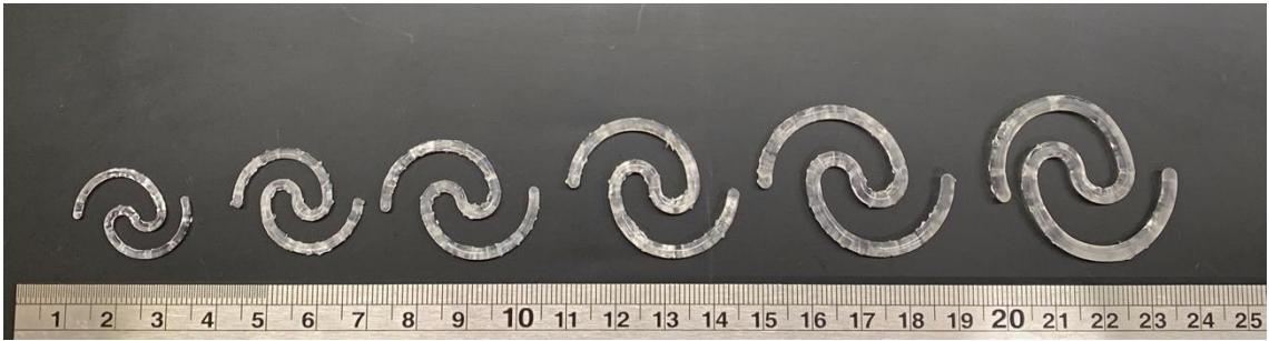
Supplementary Figure G. Photograph of the SLA 3D printed solid bladder devices in different sizes. From left to right, devices prepared with an scale factor of 0.5, 0.6, 0.7, 0.8, 0.9, and 1.0. Scale in cm.
