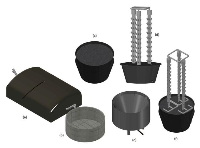
Figure 2 - Conceptual designs of the various units. (a) Anaerobic digester unit 7.5 m<sup>3</sup>, (b) Digestate storage, (c) Vermifilter unit, (d) Hydroponic unit, (e) Pyrolysis unit, (f) Combined hydroponic and vermifilter unit. The shredder is not included in this figure.
