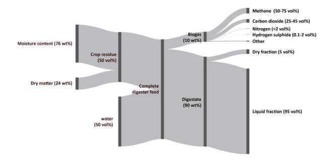
Figure 1 - Typical AD feedstock and effluent contents. Data compiled from [10], [31], [32] and [33]
