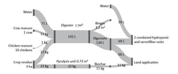
Figure 7 - Example configuration of the system with the average daily in- and outputs for a farm with 3 hectares of cropland (44 kg of crop residue per day), 10 chickens (1 kg of chicken manure per day) and 1 cow (11 kg of cow manure per day). Note that the pyrolysis unit is only used twice a month, feedstock is stored between operations.
