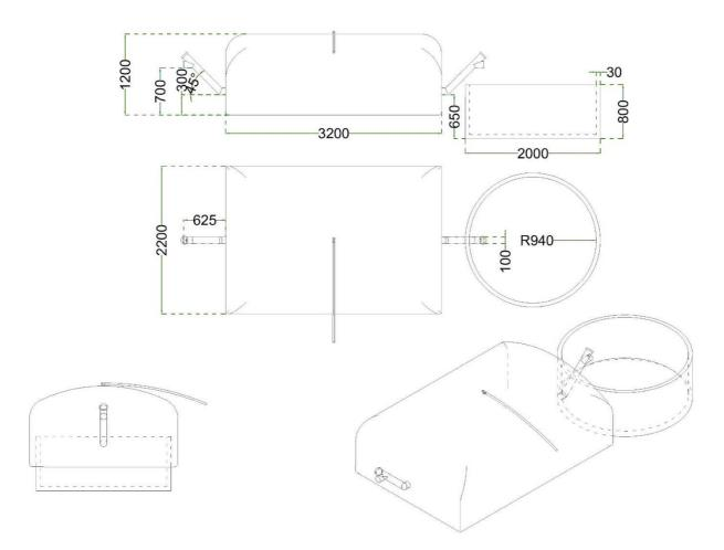
Figure S.11 - Technical drawing digester 7.5  $\ensuremath{m^3}$
