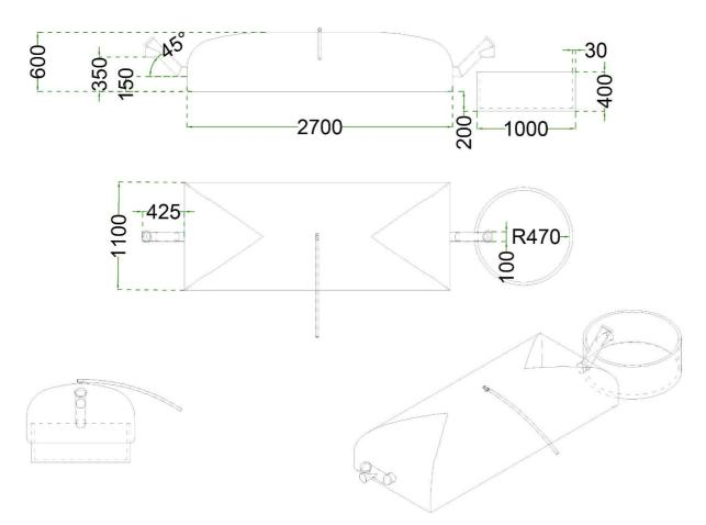
Figure S.9 - Technical drawing digester 1.5  $\ensuremath{m^3}$
