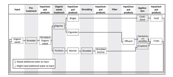
Figure 4 - System configuration with a digester 7.5 m<sup>3</sup>, pyrolysis unit and a combined hydroponics and vermifilter unit
