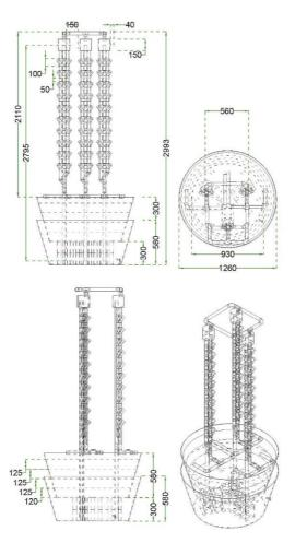
Figure S.15 - Technical drawing combined hydroponic and vermifilter unit
