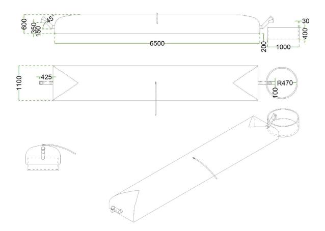
Figure S.10 - Technical drawing digester 3.7  $\ensuremath{m^3}$
