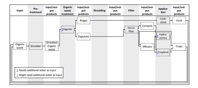
Figure 6 - System configuration with a digester 7.5 m<sup>3</sup>, a vermifilter and a hydroponics unit
