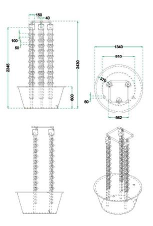
Figure S.13 - Technical drawing hydroponic unit
