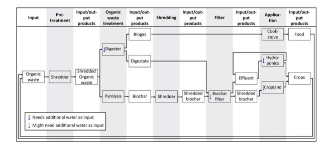
Figure 5 - System configuration with a digester 7.5  $m^3\!,$  pyrolysis unit and a hydroponics unit
