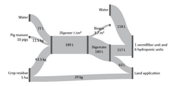
Figure 8 - Example configuration of the systems with the average daily in- and outputs for a farm with 5 hectares of cropland (72.5 kg of crop residue per day), 5 pigs (11.5 kg of pig manure per day).
