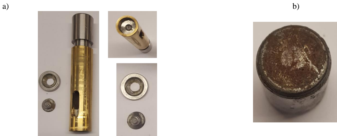
Fig. 26: a) Signs of galvanic corrosion of the BraCyl fastener b) corrosion of the central dowel pin for the SteSq prototype.
