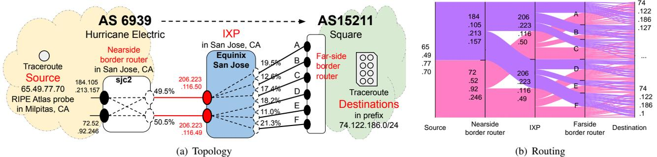
Fig. 7. Illustrations of topology and routing of a Divergent-type M-BGP deployment between AS6939 and AS15211 (Case 3 in Table III)
