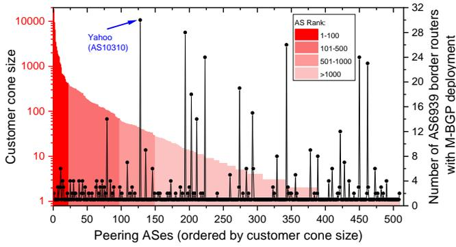
Fig. 4. The numbers of peering ASes, peering ASes via IXP, and peering ASes with M-BGP deployment at AS6939’s border routers.
