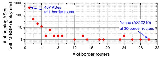
(a) Number of peering ASes with M-BGP deployment as a function of number of border routers.
