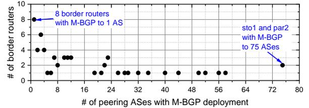
(b) Number of border routers as a function of number of peering ASes with M-BGP deployment.
