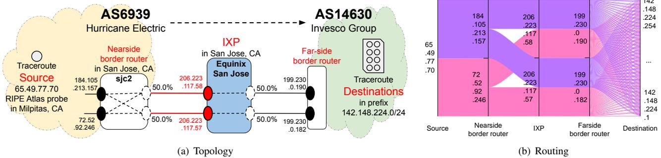
Fig. 6. Illustrations of topology and routing of a Parallel-type M-BGP deployment between AS6939 and AS14630 (Case 1 in Table III).
