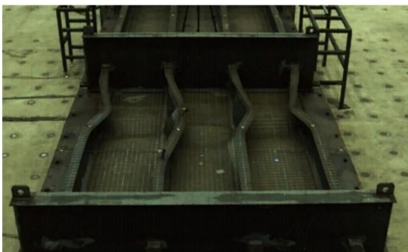
Figure 22 Deformed shape of the plate panel at the ultimate limit state observed from the experiment (Paik et al. 2020a)
