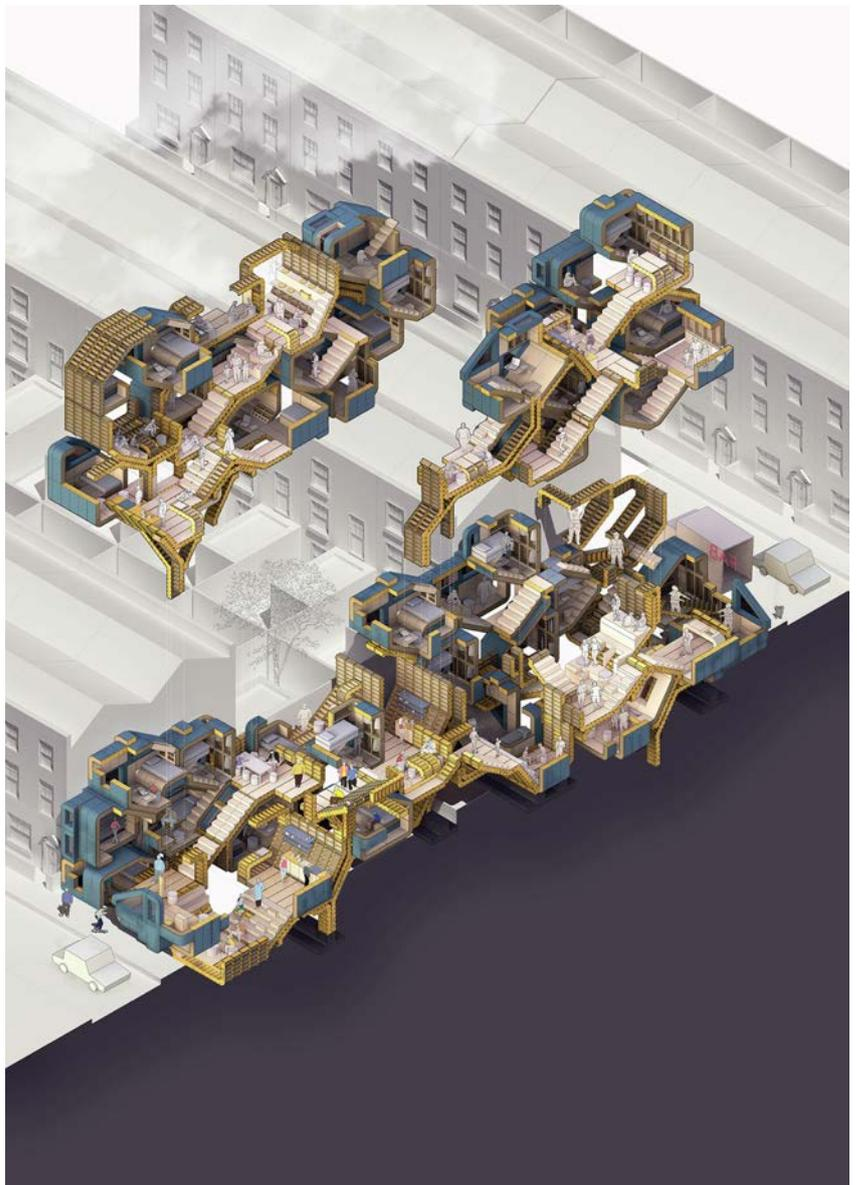
Figure 4, CNC-milled timber and cardboard discrete parts, combined to maximise privacy and shared 'living landscape', NAME OMITTED, LAB OMITTED, 2018
