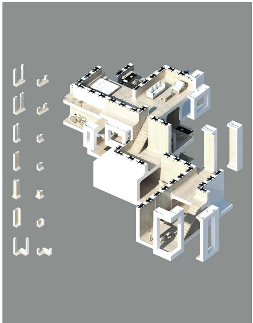
Figure 2, Spatial assembly of concrete-cast foam moulds allowing for recombination until permanent arrangement is determined by a network of stakeholders, NAME OMITTED, LAB OMITTED, 2018
