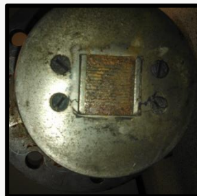
Electrodes section after a test
