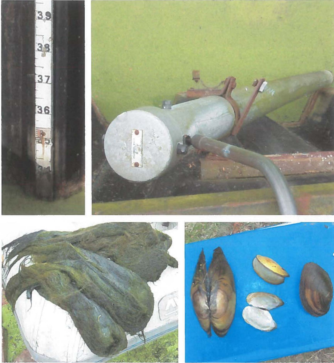
Figure 8. Photographs of stage board (top left) and broken water level gauge (top right) at sluice gate, blanket weed (bottom left) and swan mussel shells bottom right).
