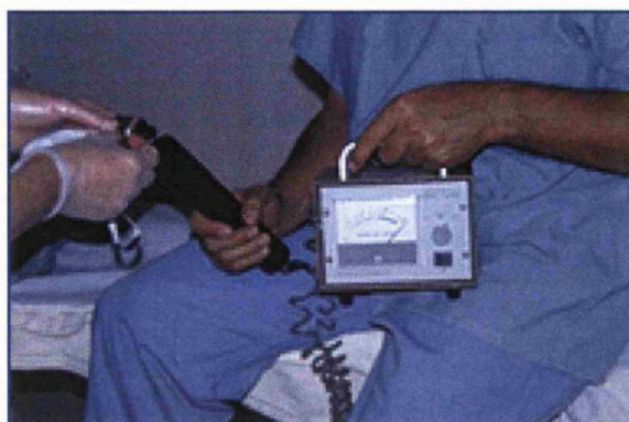
Fig 7.4 Checking operative swabs with scintillation contamination monitor
