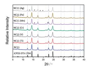
Fig. 1 XRD patterns of the as-synthesized undoped and doped cobalt-nickle sulfides, displayed together with the JCPDS pattern 073-1704 (space group Fd3m) for NiCo<sub>2</sub>S<sub>4</sub> (black). Impurity peaks for Ag<sub>2</sub>S and MnS are indicated with (\*), based on reference patterns JCPDS 014-0072 and 089-4952, respectively.
