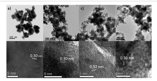
Fig. 2 TEM images of (top) and particle spacings (bottom) of the (a) undoped (NC11) (b) chromium-doped (NC11 Cr) (c) manganese-doped (NC11 Mn) (d) iron-doped (NC11 Fe) cobalt-nickel sulfide samples.
