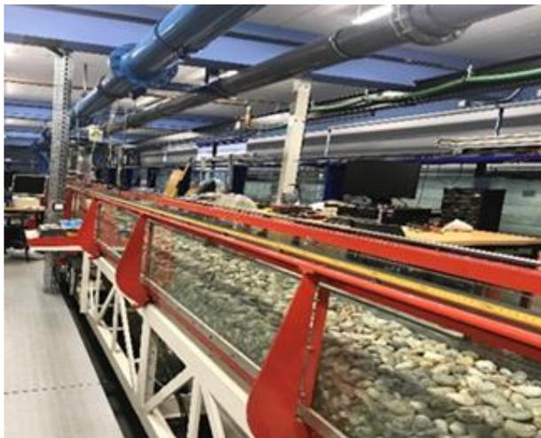
**Figure 1.** The narrow flume used in this study.
