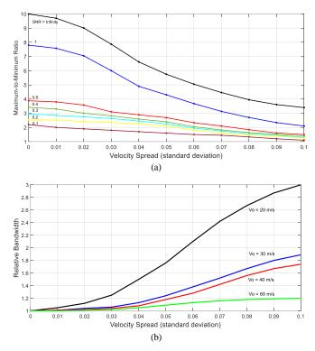
Figure 4(a) and (b). (a) decrease in max/min ratio of the delayed-andsummed output of an *N*-channel VSR system (N = 10) at the matched velocity of 30 m/s as a function of the parameter 'spread', i.e. the standard deviation of the velocity distribution. Fig 4(b) shows the increase in velocity spectral bandwidth for the same range of the parameter 'spread' (values from Fig 3(b)). Both sets of values have been normalized to for zero spread.
