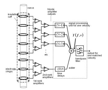
Figure 1. This shows a *multielectrode cuff* (MEC), on the left of the diagram, connected to a *tripolar* (double differential) amplifier array. The N tripolar outputs (where N is typically about 10) are delayed and added before being bandpass filtered.
