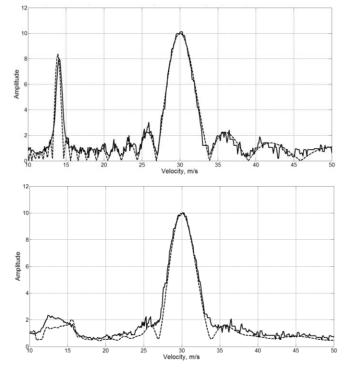
Figure 2. Comparison of time domain calculation of the velocity impulse function (VIF) of an SFAP of velocity 30 m/s with the spectrum calculated directly, for relative bandwidths of 0.1 (top) and 0.5 (bottom). Close agreement between the two is shown in both cases.
