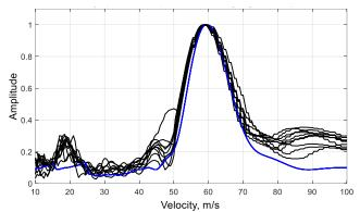
Figure 5. Measured velocity spectra taken from pig *vagus* nerve using an 11 electrode cuff connected as 10 dipoles. Ten separate runs are shown, each with the same level of electrical stimulation and with the computed VIF shown for comparison (blue trace).
