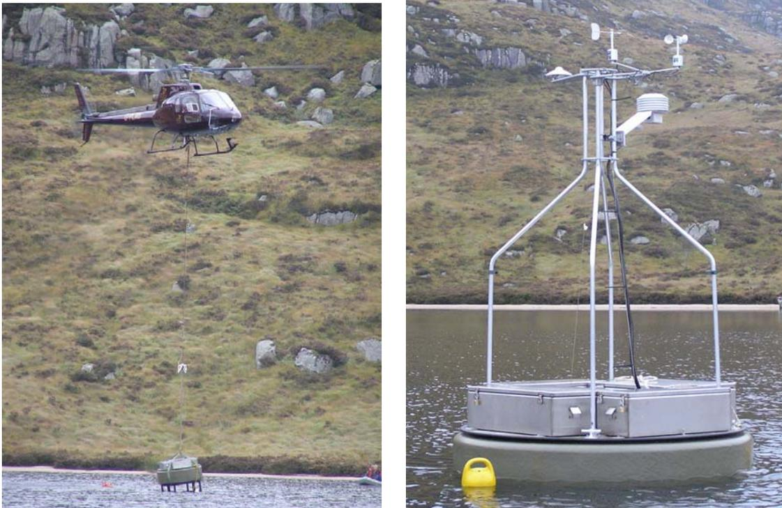
*Figure 11. a) The deployment of the AWQMS at the Round Loch of Glenhead by helicopter and b) the installed station once the sensors had been fitted on-site. (from George 2006)*
